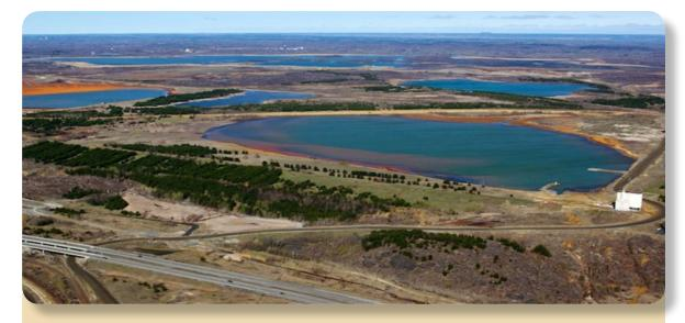
**View 3:** Aerial view of tailings ponds north of Regional Road 55 (lower left). Oxidation of the ironbearing tailings produces rusty-coloured shorelines. The slopes of the tailings pond hills have been planted with trees and grasses. *Photo courtesy of the Ontario Geological Survey.*
