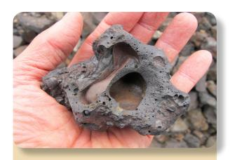
**View 6:** Fragment of slag displays a "Swiss cheese" texture that reflects its origin in a smelter furnace, where gas bubbles in molten slag were trapped as the slag began to cool to solid. Crushed slag is used as fill for the beds of roadways and railways in the Greater Sudbury area.
