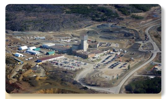
**View 7:** Aerial view of Copper Cliff (North) Mine. The concrete tower is the mine headframe. *Photo courtesy of the Ontario Geological Survey.*
