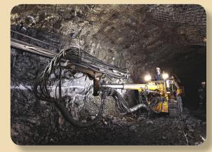
**View 2:** A rock-drilling machine used in an underground mine in Greater Sudbury. Drills mounted on the long mechanical arm are used to create holes that are then loaded with explosives. Blasting breaks the ore into rock fragments that are transported to surface and then to the mill for crushing and grinding. Photo courtesy of Vale.
