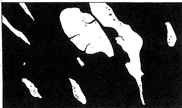
Fig. 41—Character of ore at Levaek mine, Sudbury area, Ontario, first level. Black represents sulphides; white represents granite-gneiss. Width of face 3 feet.
