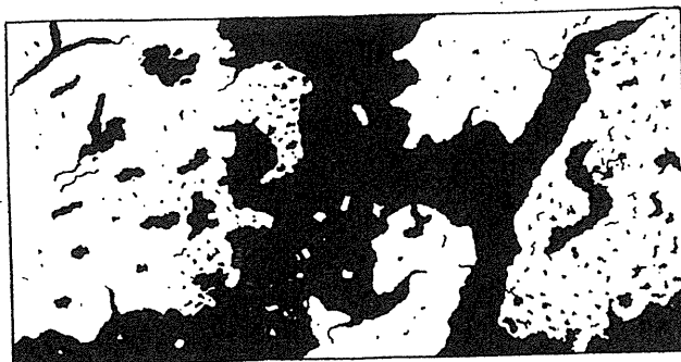
Fig. 42—Character of ore at Levack mine, third level, Sudbury area, Ontario. Black represents sulphides; white represents granite-gneiss. Width of face 1 foot. The sulphides replace or impregnate the granite-gneiss.
