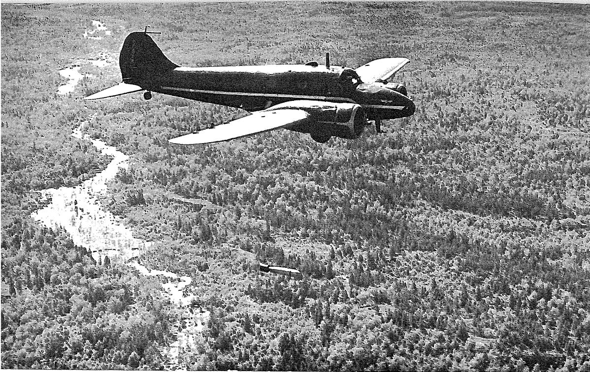
FIGURE 5. Airborne geophysical survey, magnetometer suspended beneath aircraft.
