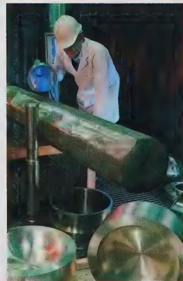
Electrostatic fluorescent dye penetrant examination of a forged INCONEL* alloy 625 bar at Daniel Doncaster. Also shown are other forged components.
