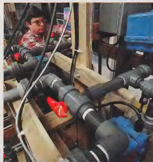
Heat transfer module is key component of Ocean Thermal Energy Conversion Project being undertaken for the U.S. Department of Energy by the LaQue Center for Corrosion Technology.
