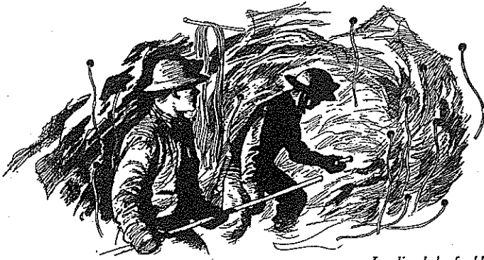
Loading holes for blasting in a drift face.
