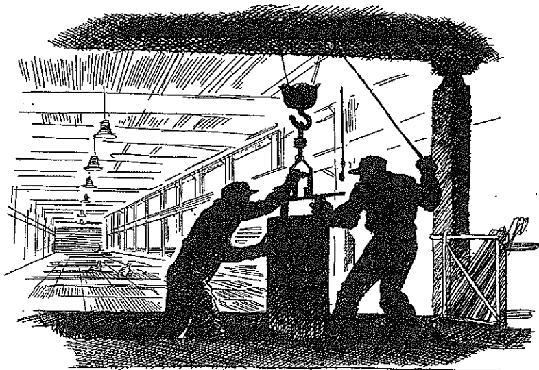
Removing nickel cathodes (99.9% pure nickel) from electrolytic tanks.
