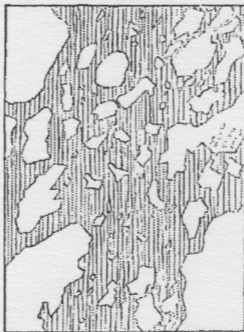
FIGURE 1—Section of brecciated ore from Murray Mine.
