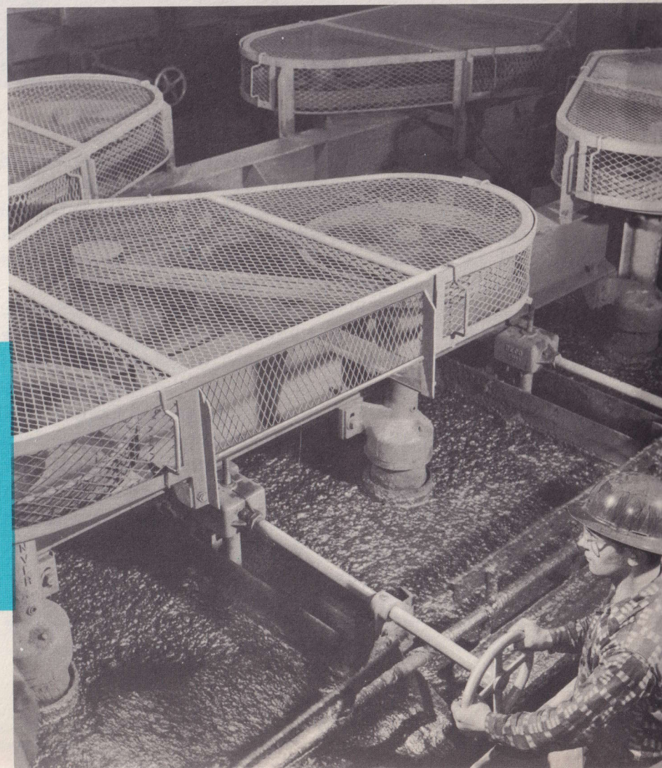
The flotation process is used to separate the ore concentrates.
